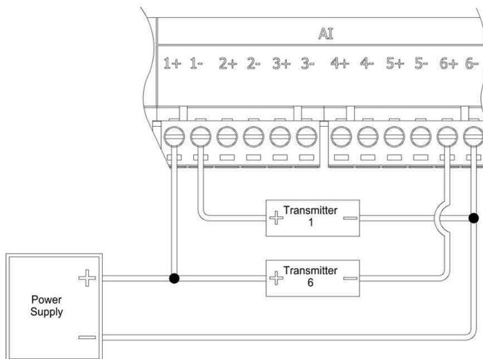
**Analog Input Wiring Example**
