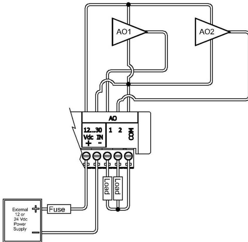
Analog Output Internal Wiring
