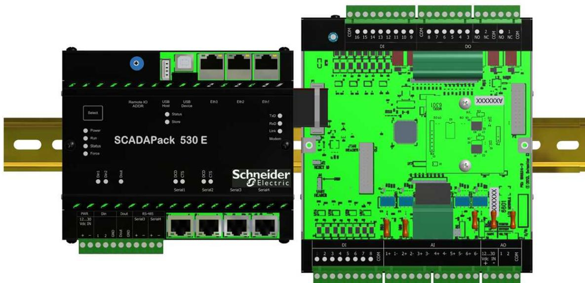
6601 I/O Expansion Module Connected to a SCADAPack 530E
