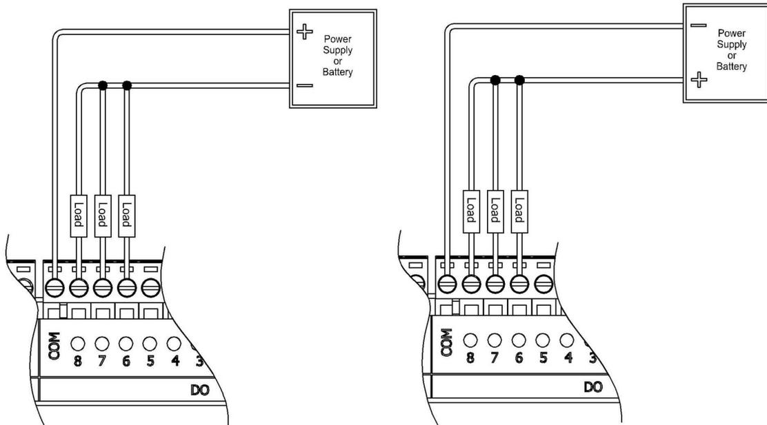
**Wiring Examples for I/O Board Form A Digital Outputs**
