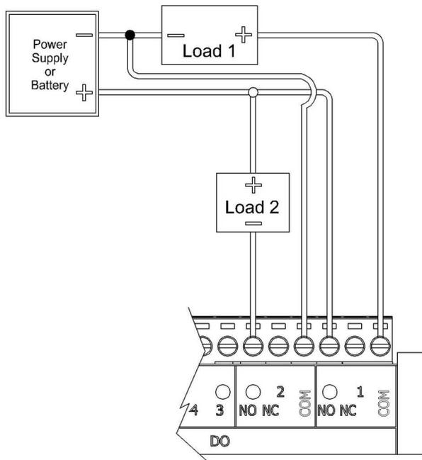
Wiring Example for I/O Board Form C Digital Outputs
