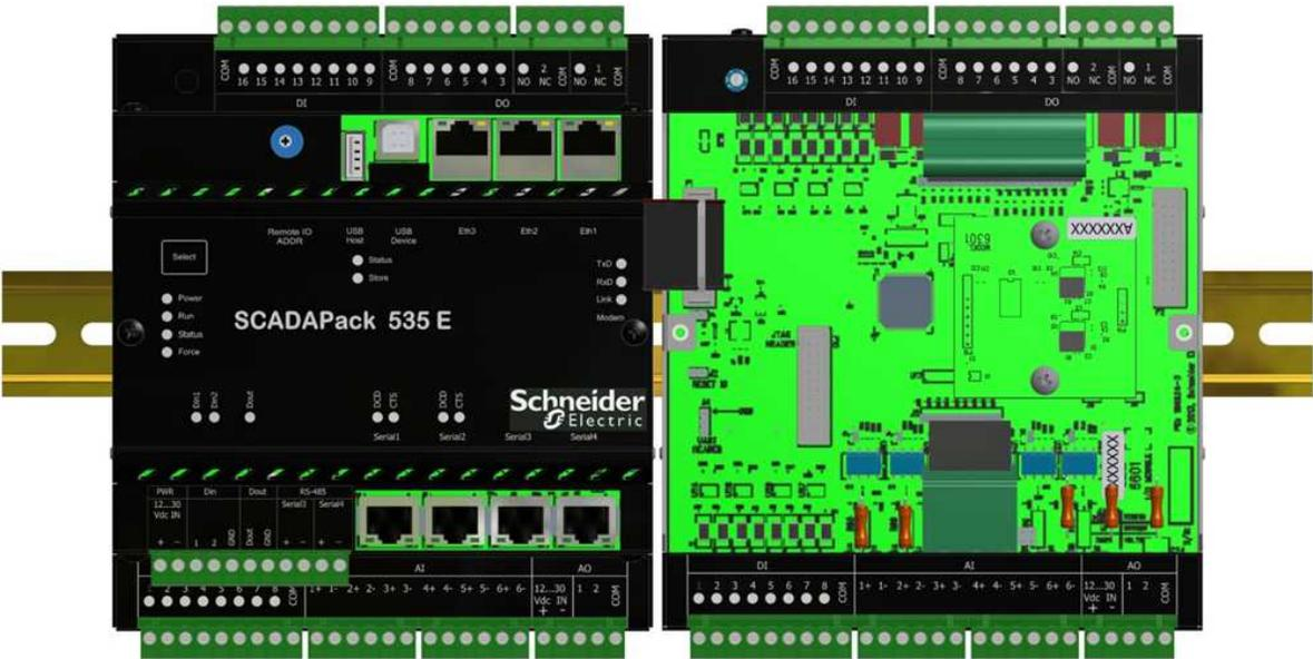
6601 I/O Expansion Module Connected to a SCADAPack 535E
