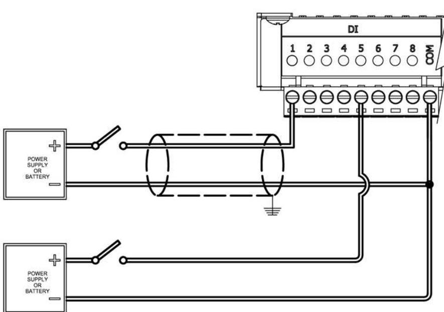
**I/O Board Digital and Counter Input Wiring Example**
