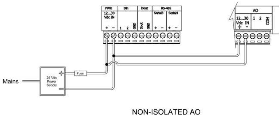
**Power Supply Configurations for Isolated and Non-Isolated Analog Outputs**
