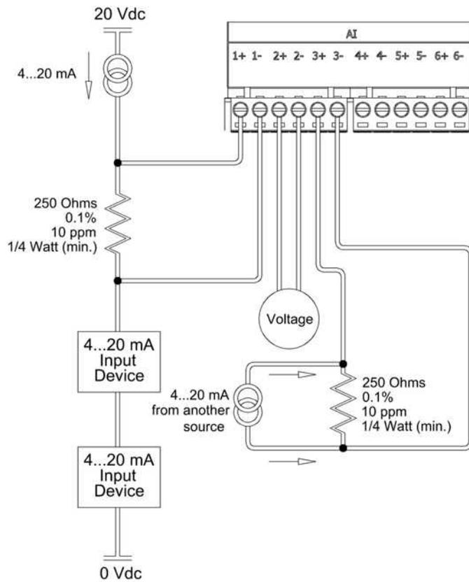
**Wiring to Support a Mix of Current and Voltage Inputs**
