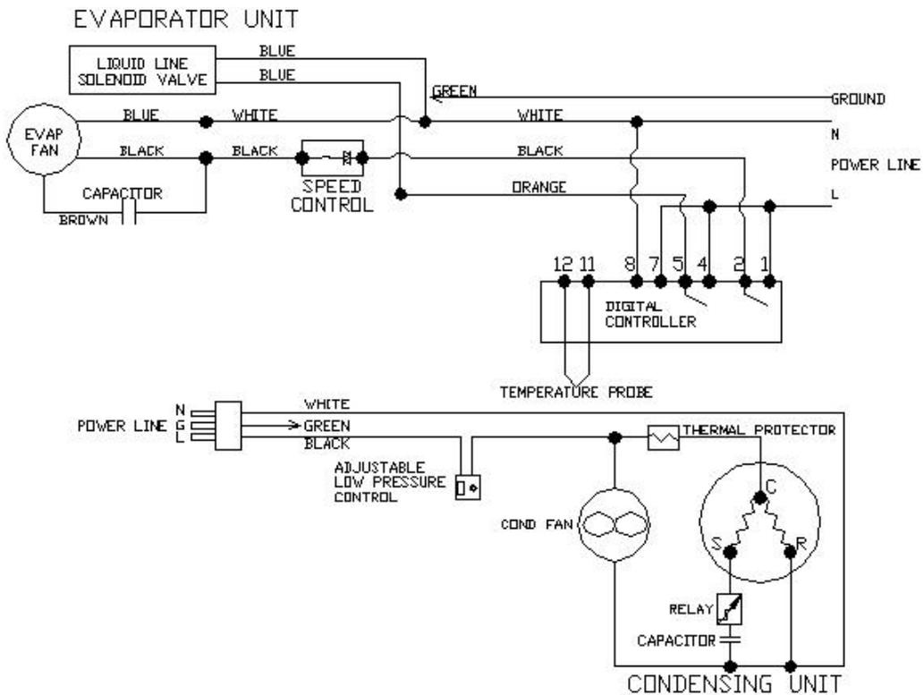
**Fig. 2.5 VINO650SSR Electrical Wiring Diagram (DIGITAL CONTROLLER)**
