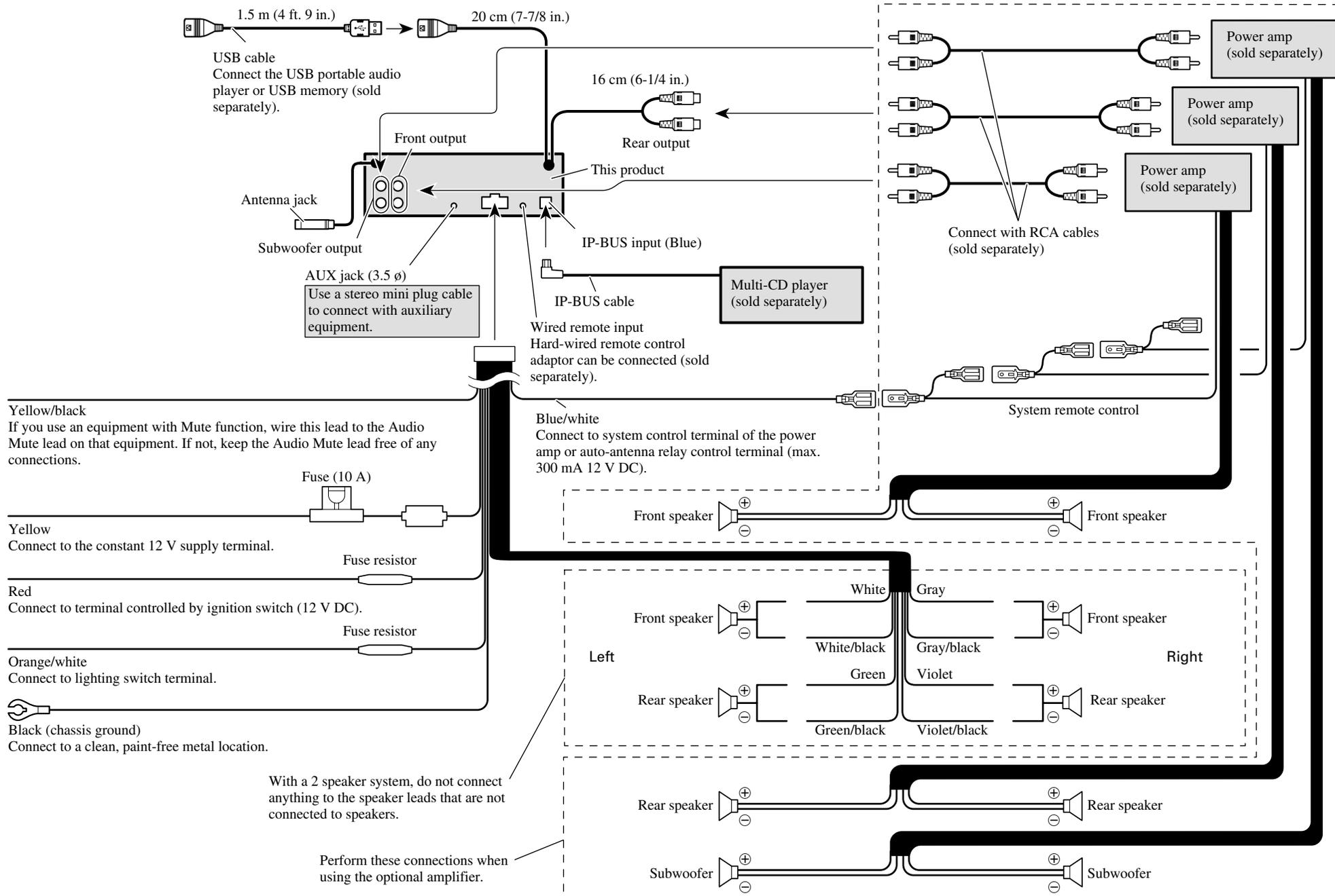
■ When using a Subwoofer without using the optional amplifier
