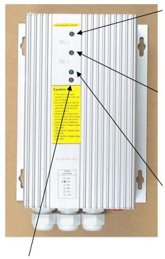
**Power light**: If everything is operating properly this will be green. If it is not green then the voltage may be too low (not enough sunlight), the pump is drawing too much current (head too high) or the controller temperature is too high (put it in a cool position with plenty of air circulation).
