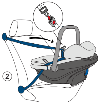
Picture 2: Click the car seat belt into the car seat belt lock. Make sure that it clicks into place with an audible "click".
