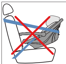
Picture 6: Tighten the seat belt hard and make sure that it is not twisted in any place. Make sure that the seat belt is correctly tightened through the blue belt movers by the baby's pelvis and behind the head barrier.
