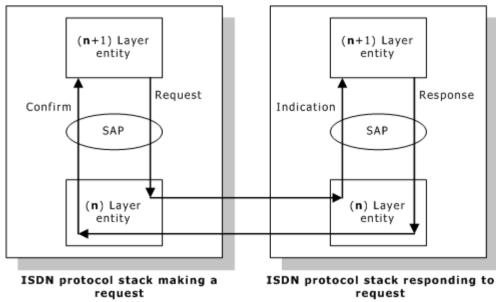
Four types of primitives are exchanged between adjacent layers:
