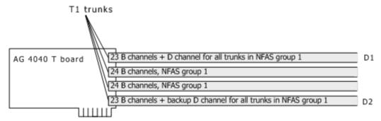
At any point in time, only one of the D channels, D1 or D2, conveys B channel signaling information. The other D channel remains in a standby role and is active at the LAPD layer (layer 2) only. While the backup D channel is on standby, any layer 3 messages received on it are ignored.
