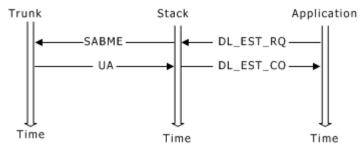
If the SABME message is not acknowledged (the physical link is down, or the remote equipment is not prepared to complete the link), the stack sends the SABME message four more times, at one second intervals. If the message is not acknowledged within five tries, the stack sends a DL\_REL\_IN message to the application. NMS ISDN remains in the IDLE state.
