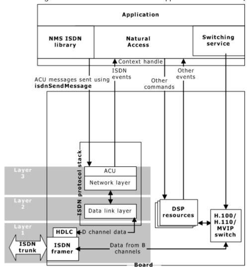
The following illustration shows the NMS ISDN application architecture (ACU configuration):
