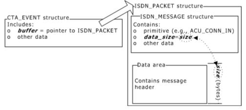
After receiving and processing the data within the CTA\_EVENT event buffer, the application must use **isdnReleaseBuffer** to free the buffer as quickly as possible. Otherwise, the ISDN interface times out and stops passing events to the application.
