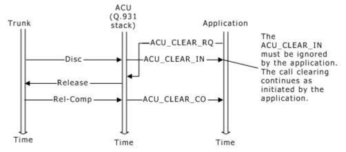
Clear collision at the network level takes place when a DISCONNECT message is received by the network directly after it sends a DISCONNECT message to the stack. The following illustration shows the sequence of messages exchanged in this situation:
