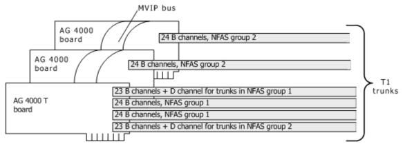
If the application uses NMS ISDN in a channelized configuration, all trunks in an NFAS group must be on the same board. An NFAS group cannot contain trunks from multiple boards. This restriction does not apply to the ACU configuration or the LAPD configuration.
