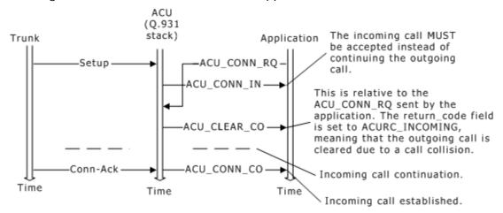
The ACU\_CLEAR\_CO message is relative to the ACU\_CONN\_RQ sent by the application. The return\_code field in the primitive's message data is set to ACURC\_INCOMING, meaning that the outgoing call is cleared due to a call collision. No answer is sent by the application in response to this ACU\_CLEAR\_CO message.
