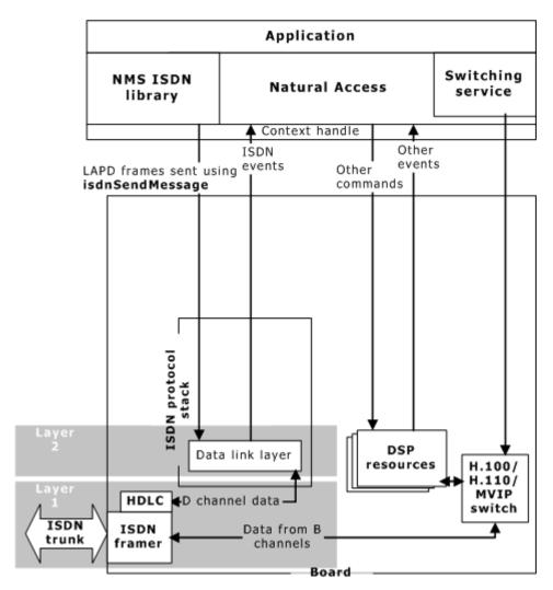
In this mode, the protocol stack implements ISDN layer 2 functionality. No ACU is present. Instead, the application uses the NMS ISDN Messaging API to send LAPD frames directly to the data link layer (layer 2).
