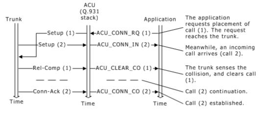
If the ISDN stack is configured as network equipment, it continues with its call setup attempt, signaling the trunk to release the incoming call. The following illustration shows the sequence of messages exchanged in this situation:
