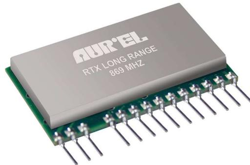
RTX-LONG-RANGE-869MHz radio transceiver half-duplex, offers improved performance, as such as longer RF range up to 3Km, operates in European band 869,4÷869,65MHz free licensed with no government taxes. The high sensitivity level (-118dBm) joined with its typical ERP (+27dBm) can assure a budget-link around 145dB, improving communication distance of 4-5 times better compared with traditional 10mW LPD devices.
