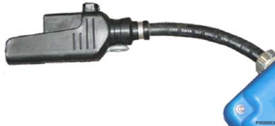
Figure 2: Trainline Interface (Inter-Car Cable)
