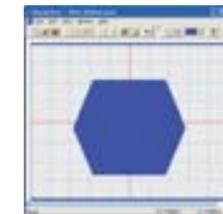
② After loading the mask pattern to DL9000 MSO models, you can perform error rate analysis or go/no-go judgment.
