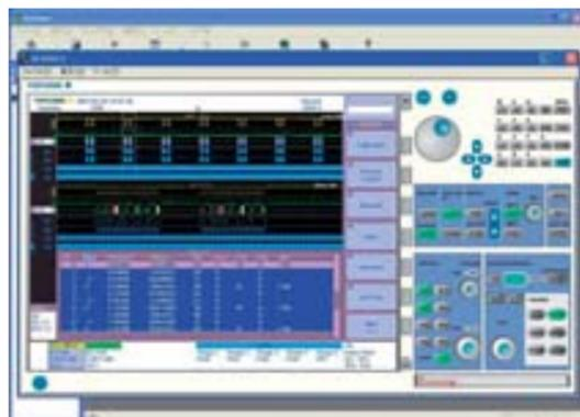
Control a DL9000 MSO model via USB or Ethernet. Provides simple control and transfer of waveform data to a PC through an intuitive man-machine interface.
