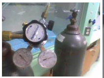
CO2 Tanks & Regulator
