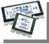
Figure 2.7 12V, 100W - 15V, 75W dc to dc converter VI - 200. This picture has been obtained from the official website of Vicor corporation.
