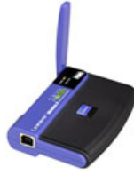
Figure 2.5 WUSB54G an 802.11g standard USB based W - LAN network adapter card. This picture has been taken from the official website of Linksys Inc.
