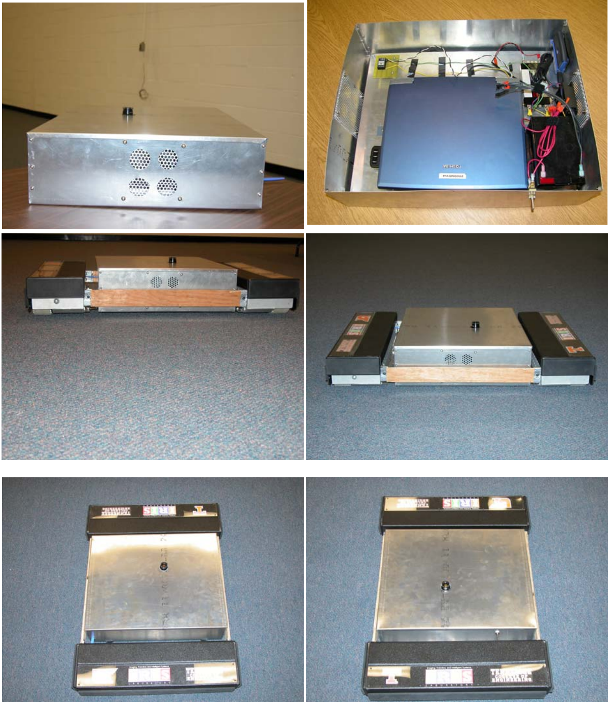
Figure 3.6 Different views of the packaged infrared imaging sensor brick mounted on the tracked under vehicle robot.
