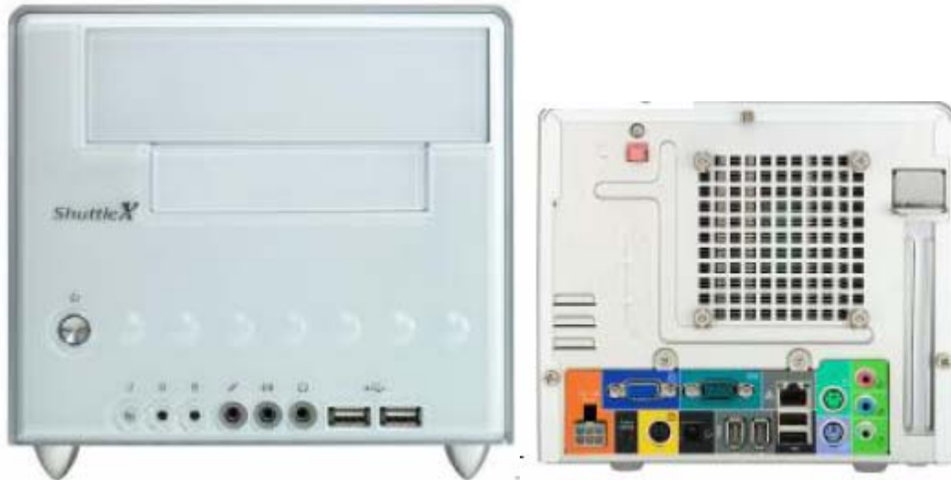
Figure A.2 The front and back panels of the Shuttle PC respectively. This was the CPU for our revised version of the design.
