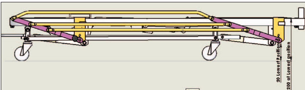
Figure 1: Low Height Clearance
