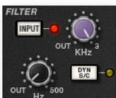
The Filter controls provide access to two separate kinds of filters. The black knob controls an 18dB/Octave high-pass filter (20Hz to 500Hz). Use it to remove lower frequencies from the audio. The purple knob controls a 12dB/Octave low-pass filter (3kHz to 22kHz). Use it to remove higher frequencies.
