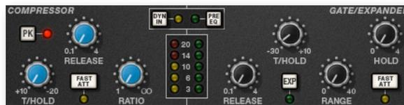
**Noise Gate/Expander:** To activate the Noise Gate/Expander, turn the Range knob so that its range is no longer zero. The green indicators in the right-hand of the two meters in the centre of the Dynamics section show the amount of gain reduction being introduced.
