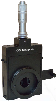
Micrometer adjustable slit assembly. The slide shown on the right is used to adjust the height and the micrometer adjusts the width of the slit. Note that the input and output slits should be set to the same width and height.
