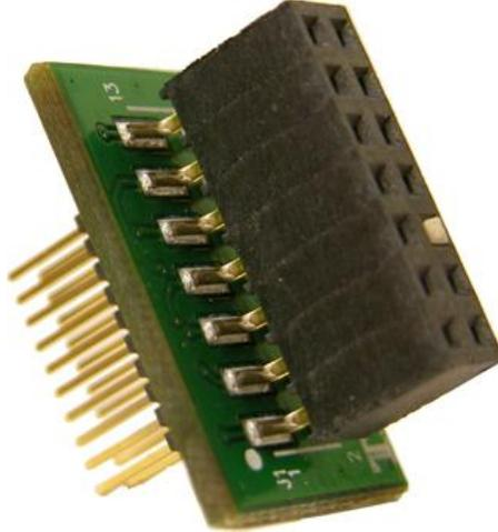
**Figure 71. JTAG 14 to 20 Pin Adapter**
