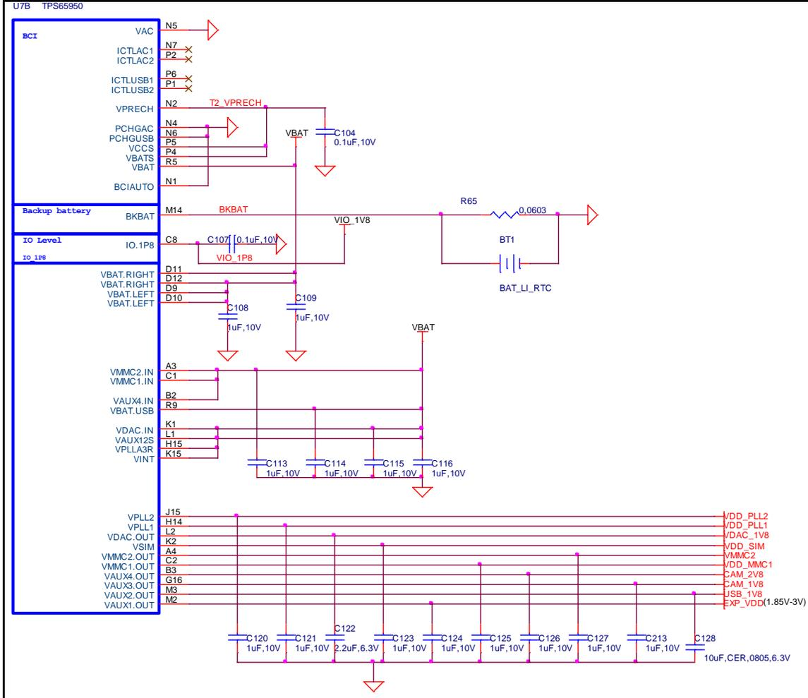
Figure 26. Peripheral Voltages
