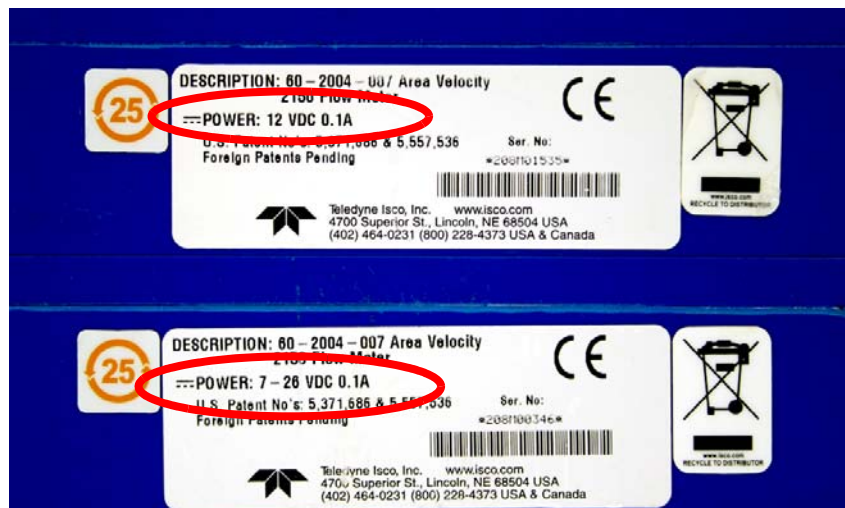
Figure 2-3 Identifying the 2150 voltage specification
