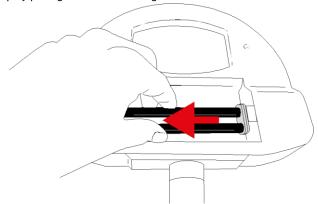
Align the pins at the end of the lamp with the slots in the fitting
