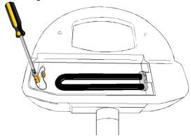
Expose the lamp below by lifting the lamp protection cover and sliding it out of the retaining slot.
