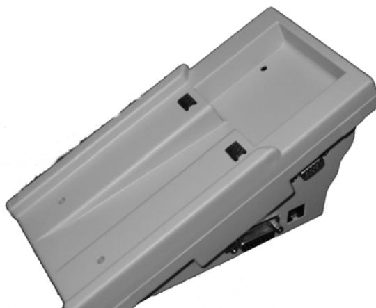
The base unit accommodates the Terminal Unit. The communication between the TU and the Base Unit is through mating connectors on the back of the TU and on the top of the BU. An External PTT is connectable to the side of the BU. External power can be connected to the BU by a regulated AC-DC adaptor (Not included) connected to 120VAC 60 Hz input, providing to the BU its 7.5 VDC 500mA output .
