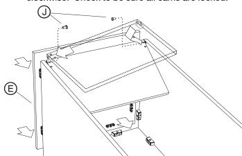
Turn the cabinet onto its left side. Tap the N Door Hinges into the recesses on the Large Door. Fasten using N Screws through the hinge leaf and into the pre-drilled holes. Use N Screws to fasten the M Door Hinge Mount Plates onto the left panel, through the hinge leaf and into the pre-drilled holes.
