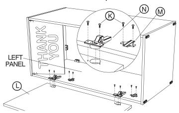
Bend the arm of the Hinge and slide the arm into the Hinge Mount Plate. Set the Waste Receptacle upright. Center the Lower Door panel by adjusting the set screws on the Door Hinges either in or out as needed.
