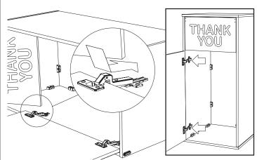
Adjust the Upper Door vertically so it does not brush against the Lower Door panel. Do this by loosening the screws on the hinge plates, and repositioning the panel. Re-fasten all screws. Place the Plastic Liner (model 9669, sold separately) in the cabinet.
