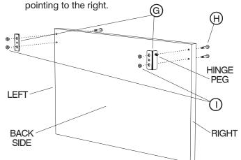
Press the J Plastic Inserts into the small hole near the upper end of each side panel. Carefully tilt the F Small Door until the Hinge Plate pegs can be inserted into the Plastic Inserts.
