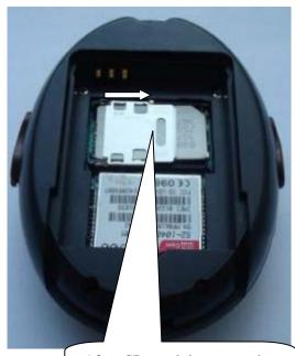
After SD card is mounted, Fasten the simcard rightwards
