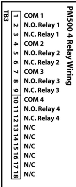
**Figure 3; 6 Relay outputs wiring diagram**
