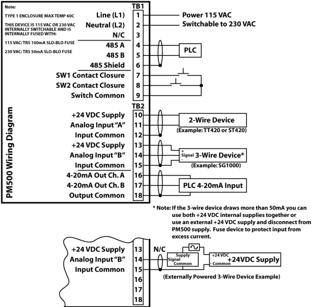
Figure 1; PM500 Wiring Diagram
