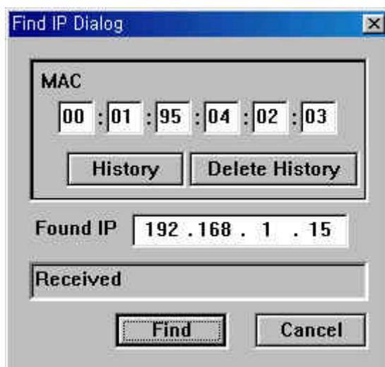
**Figure 4.10 IP address check using the [IP Find] function**
