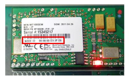
Figure 4-18 Locating the NODE ID (MAC address) on the ethernet modem
