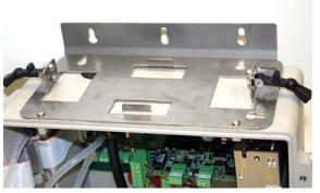
Figure 4-6 Installing the battery backup mounting plate
