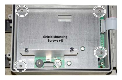
Figure 5-4 Remove non-bubbler shield
