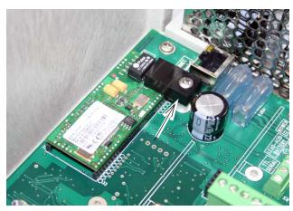
Figure 4-16 Ethernet modem installation
