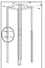
**3)** Extend the angle bars to the required height and then fix them in position using the 16 x M4 nuts and bolts with metal washers.
