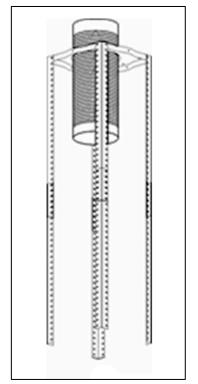
**4)** If your cooker hood is going to be used in extraction mode, then you should connect the ducting hose to the ceiling adaptor at this point.
