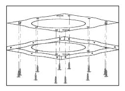
**1)** Position the hanging plate on the ceiling and then mark the position of the screw holes.
