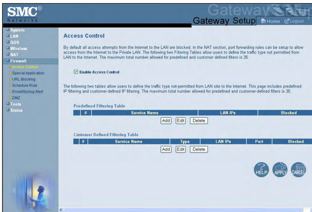
Figure 40. Access Control Menu
