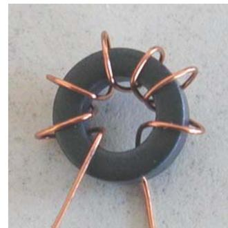
[ ] Tr.2 FT50-43 primary 4 turns isol. mounting wire, secondary 7 turns 0,5mm copper wire on the larger black toroid.
