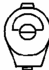
If a trimmer has reached its maximum, the only solution is to remove the corresponding coil and re-wind it with an extra turn. If the trimmer is at minimum, you will correspondingly have to remove one turn.
