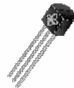
Many small signal transistors and voltage regulators are made in TO 92 cases. The component placement drawings show all components basically from above. When mounting, please note the direction of the rounded part of the casing. Please do not mix up the two voltage controllers, which are both in TO92 (the 8 V regulator is marked L08, and the 6 V regulator marked L06). Voltage regulators like these look
