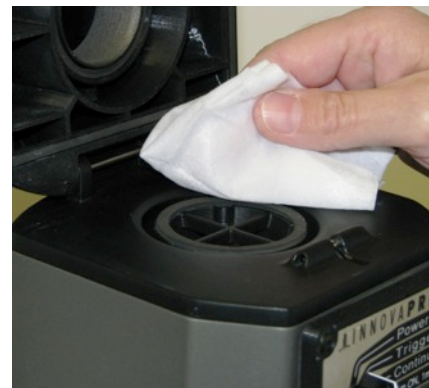
FIGURE 4.22 CLEANING INTERIOR SURFACES
