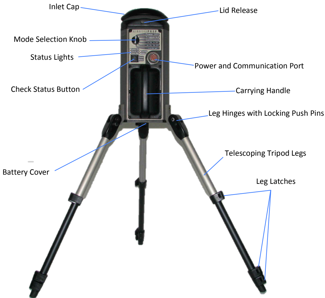
FIGURE 3.1 COMPONENTS OF THE ACD-200 BOBCAT
