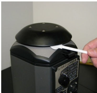
FIGURE 4.21 CLEANING INLET WITH FOAM TIPPED APPLICATOR
