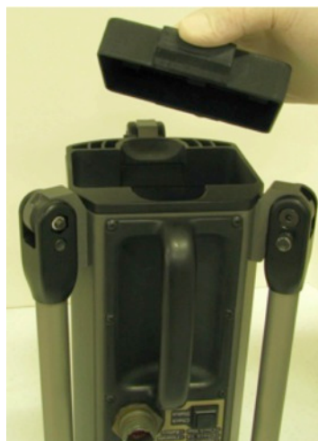
FIGURE 4.10 REMOVING BATTERY COVER
