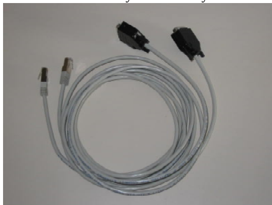
DB15 to RJ 45 cables.
