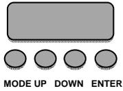
Browse through the menu by pressing Mode. You can change the selection by pressing Up or Down. Press Enter in order to confirm. You can leave every mode by pressing Mode. The functions provided are listed in the following sections.
