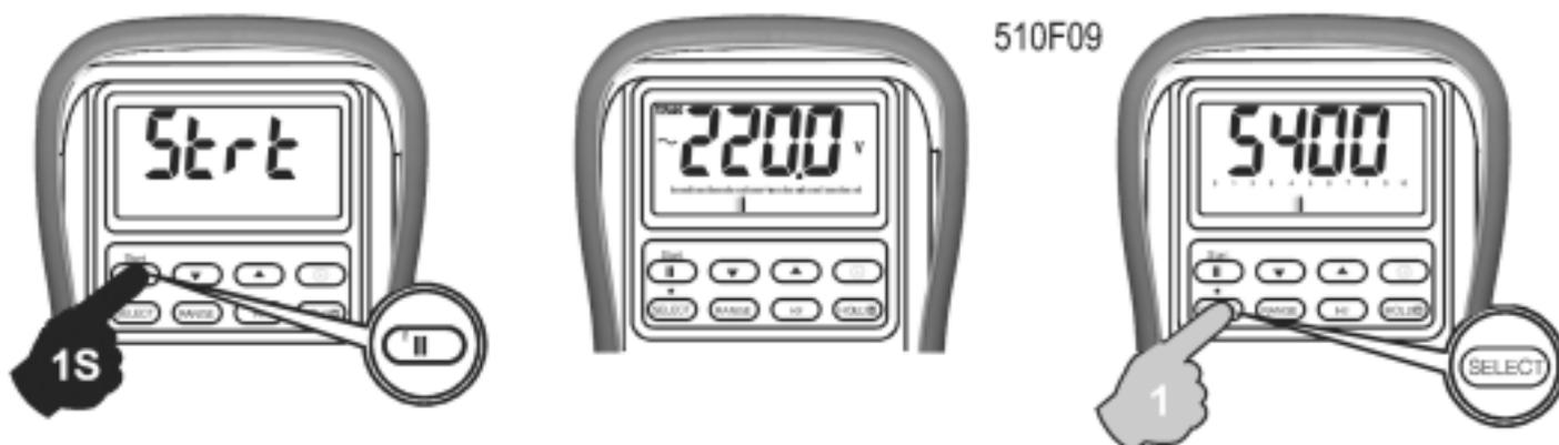
Press the **Start** button momentarily to pause or to continue. The LCD annunciator “H” will be flashing when paused.
