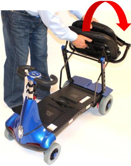
6. Grab the strap that is located in the middle of the floorboard and pull up while pushing the seat down.
