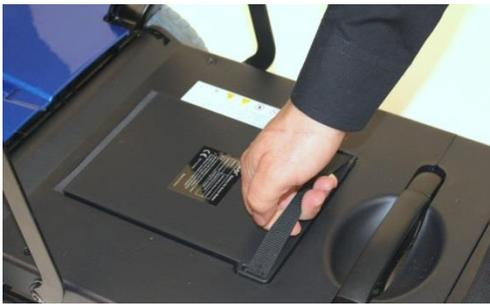
2. Pull up until the cartridge is dislodged. Be careful not to hit your hand on the bottom seat metal bar when pulling up. Repeat the same steps for the battery.
