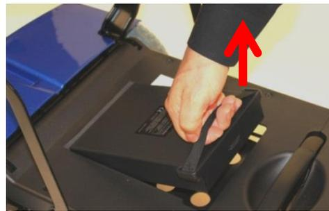
3. Swap the battery with the “dummy” battery cartridge as the label in the middle of the floorboard illustrates.
