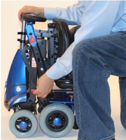
2. Carefully grab the control panel or tiller handle and push the Mobie forward while holding the seat.
