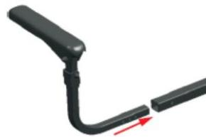
2. Secure the armrest as shown using the hardware that is included.
