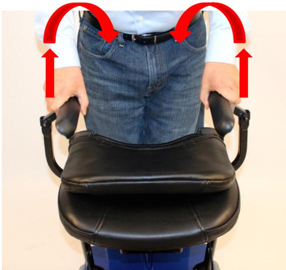
4. Push in the "Seat Lock" handle that is located under the seat while holding the rear of the seat. This allows the seat to start the accordion-like fold.
