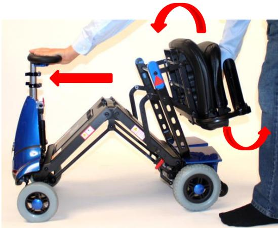
4. As the scooter unfolds, either push the floorboard down with your hand (avoid pinch point) or place your foot on the floorboard and press down until it locks in place. Do not place your foot in-between the "Pinch" point of your foot may get injured.
