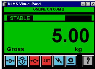
This PC software is single user purposed. Measurement on LCA device can be monitored and also all changeable parameters on the device can accessed (scaling, calibration, communication format and parameters, unit selection, optional setups etc.). **Dlms\_VP** software can communicate with only one LCA device. If there is an RS485 bus then **Dlms\_VP** can connect to each device on the bus separately.
