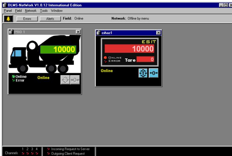
**Dlms\_NW** communicates with more than one device and can setup all user changeable parameters on each device. This PC software shares own data with other computers on the Network. According to this, each device on the system, even connected on the different computers, can be displayed on every computer.
