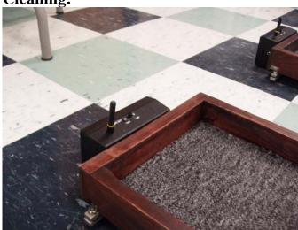
All of the electronics boxes relatively are sealed against moisture; therefore a damp cloth should be acceptable for cleaning the plastic boxes. On the display unit, Windex or some other window cleaner should be used to keep the plastic window for the LCD clean. The rail carpet can be cleaned with a normal vacuum cleaner without affecting the load cell performance. The wood siding on the rails can be cleaned with any typical wood cleaner.
