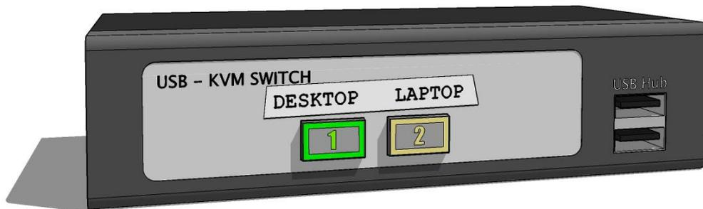
3. Press the **Laptop 2** button on the **KVM Switch Box**. The image from the laptop or other device will be projected through the classroom's **LCD PROJECTOR**.
