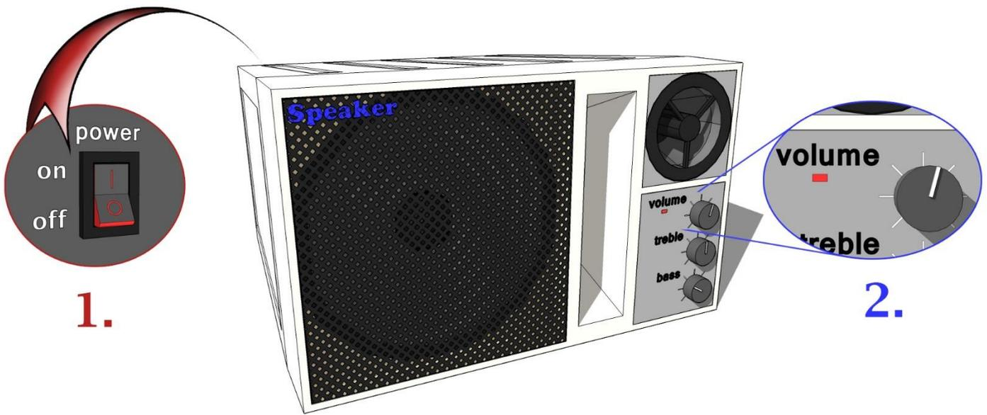
1. To **turn on** the speaker, flip the **On/Off switch** on the back of the speaker. A red light on the front of the speaker will light up to indicate that the speaker is on.
