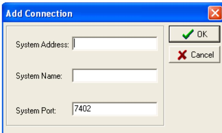
The system address can be a host name, or an IP address. The default system port is 7402.
