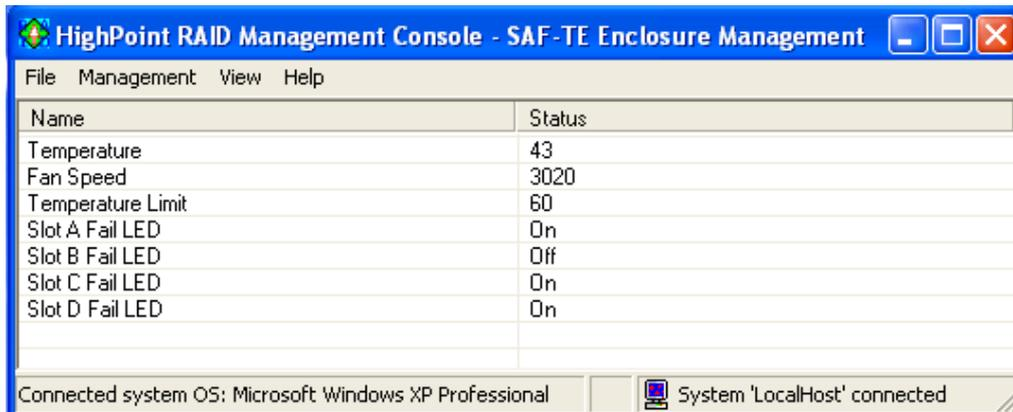
This feature allows the administrator to view and monitor a variety of SAF-TE related attributes, such as chassis temperature readings, disk failure, and the status of the chassis cooling apparatus (cooling fans).
