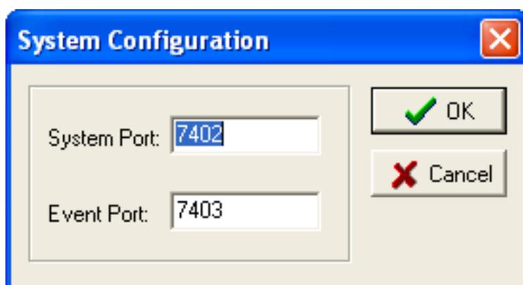
**System Port** - This is the TCP port number that the RAID Management Service uses to communicate with RAID Management Console. When you connect to the service, the port value you enter must be in accordance with the system port value on the service. The default value is 7402.
