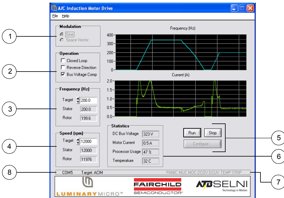
Figure 2-1. AC Induction Motor Main GUI Window
