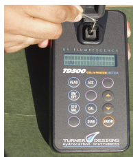
Picture 3. Adjusting the value on the CheckPOINT™ Solid Reference Standard by turning the attenuation screw.
