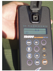
Picture 2. Placing the adjustable CheckPOINT™ Solid Reference Standard in the TD-500™.
