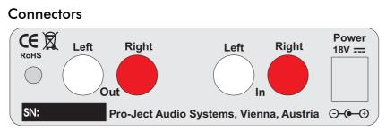
Make all connections whilst the phono amplifier is disconnected from the power supply.
