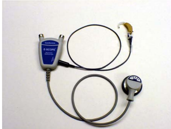
E-Scope with DAI cable connected to audio shoe (boot) of a BTE hearing aid.
