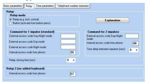
Relay mode – the relay can be preset into 2 different modes
