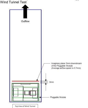
Airflow Speed Requirement Downstream of the Pluggable Module in Wind Tunnel Test • Ventilation Grille on the Display Back Panel
