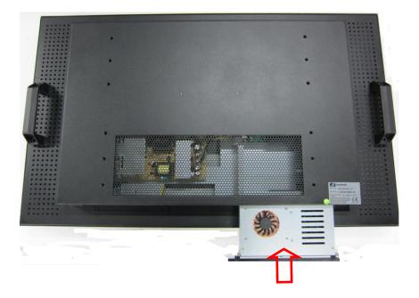
Step 4 Secure the cover by using the two screws from step 2
