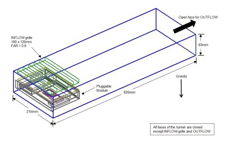
Wind Tunnel Test for the Pluggable Module
