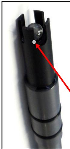
ORP is measured as the voltage drop across the platinum membrane of an ORP electrode. A reference electrode is used to complete the voltage-measuring circuit. Because platinum does not react with ions in the water, it won't give or take any electrons from those ions unless they are very persuasive. The potential (voltage) created by this refusal is what you're actually measuring as ORP.
