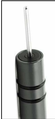
The Temperature sensor is an electrical resistor (thermistor) whose resistance changes predictably with temperature. The sensor is protected by a stainless-steel tube. Thermistors are very stable with time and do not require calibration.
