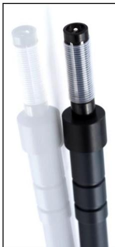
The TDG sensor is a pressure transducer (the same one used for the 10-meter depth sensor) attached to a “membrane”. This membrane is a long piece of thin-wall, silicone tubing whose job is matching gas partial pressures inside the tube with those of the surrounding water. The sum of those partial pressures is measured by the transducer, and that’s the TDG of the water.
