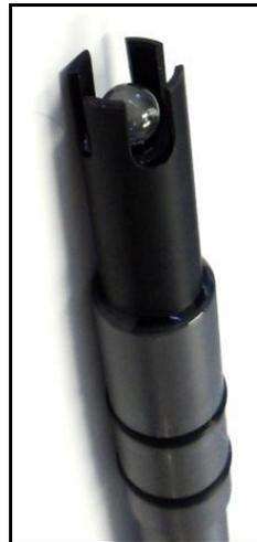
measuring circuit. The pH glass is specially formulated to absorb water so that ions (particularly H<sup>+</sup> and OH<sup>-</sup>) in the water are attracted to the glass to offset the ionic constituency of the pH electrode's internal electrolyte. As a result, there is a charge separation across the glass, and that's the voltage we measure. pH readings are automatically compensated for temperature.
