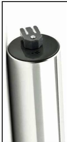
material that accumulates on the optical surfaces of the Turbidity sensor is indistinguishable from material in the water, so most Turbidity sensors have little wipers to clean the window(s).
