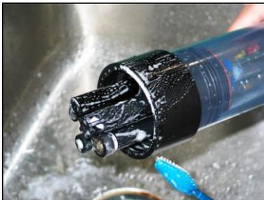
Clean your instrument periodically with warm soapy water. Liquid dishwashing soap is fine. Do not use abrasives. Do not use acetone. Do not clean with gasoline, kerosene, or industrial cleaners. Mild household cleaners work well. Clean sensor stems with a soft brush.
