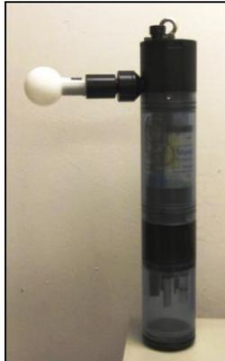
The PAR (photosynthetically active radiation) sensor measures the amount of light available to biota for photosynthesis. Its units of measurement are micro-moles of photons per square meter per second, or photon  $\mu\text{moles}/\text{m}^2$  second. This is also referred to as micro-Einsteins per square meter per second.
