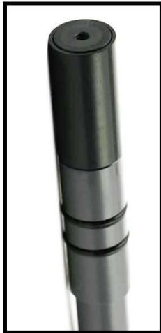
Depth sensors require no regular maintenance, but you might check occasionally to make sure the pressure port (i.e. hole in the front of the housing's bottom cap or the sensor's cap that has no apparent use) is not clogged. If it is, do not attempt to unclog it yourself; call the factory for instructions.
