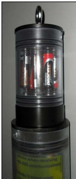
The 2-, 2.5-, and 3-inch Manta 2's, and the Sub2 and Sub3 Manta variants, use the optional Manta 2 External Battery Pack (EBP): a watertight (to 200 meters) housing with a cassette for eight "AA" batteries and a data port. Remove the EBP to connect your Manta to a PC for dumping logged data, or for calibrating the Manta sensors.
