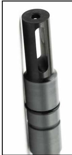
MEAS uses the four-electrode method to determine water conductivity. Two pairs of graphite electrodes are situated in a stable geometry (you can barely see the electrodes; they look like two bull's eyes inside the slot on the conductivity sensor).
