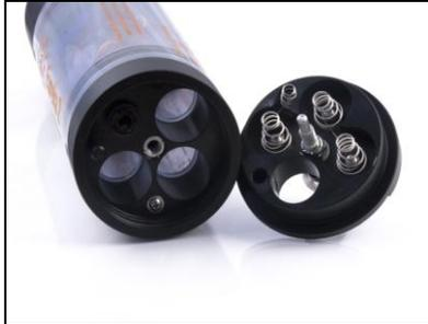
Here are Manta 2's with the switch plate set to OFF, the switch plate removed, and with the switch plate set to ON.
