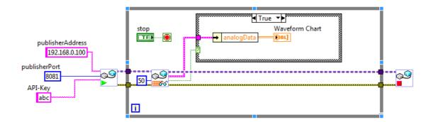
With Three Vis, a client connects to a server, providing the required API-Key, displays received analog data packages, and close connection when task is over. The above example illustrates that SCCT programming style is perfectly integrated in LabVIEW, easy to debug and maintain.
