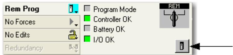
**Tip:** For 1756-L7x controllers only, *Energy Storage* instead of *Battery OK* appears beside the **Controller Properties** icon. See the [ControlLogix System User Manual](#), publication [1756-UM001](#) for information on the Energy Storage Module.
