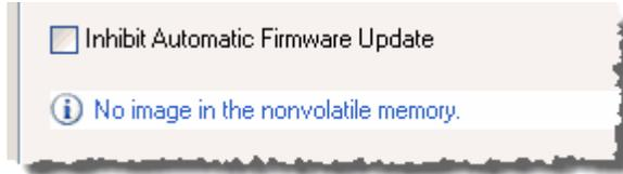
5. At the bottom of the **Nonvolatile Memory** tab, select **Inhibit Automatic Firmware Update** checkbox if you do not want to automatically store an image during a Save or Load operation.
