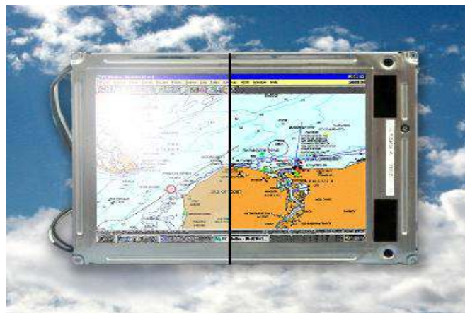
Figure 4 – Comparison with and without Optical Bonding
