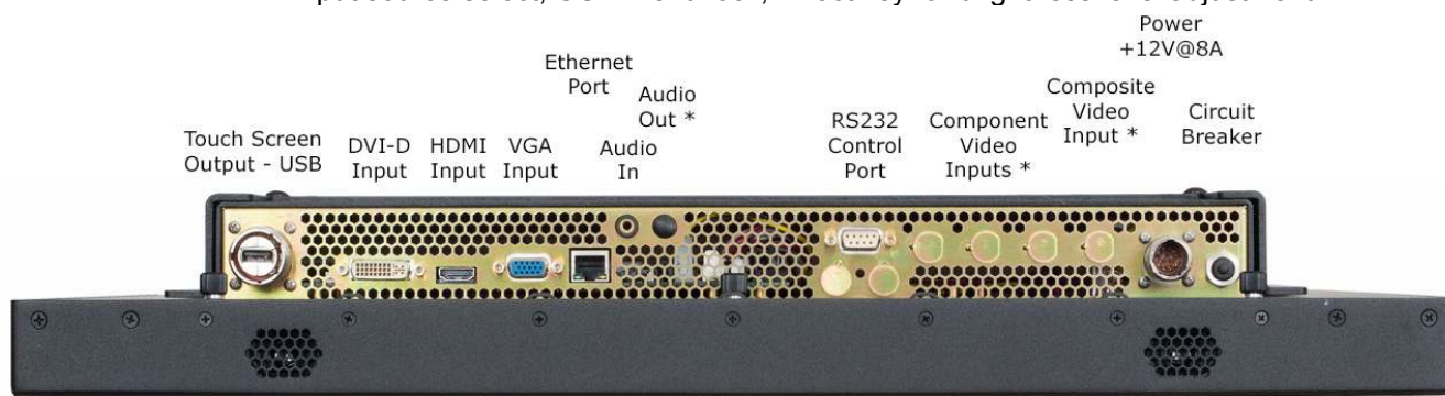
Photo 2 – Standard Controller Rear Panel I/O
