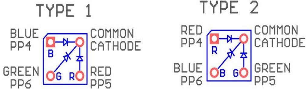
The Common Cathode RGB LED comes in two different pin configurations as shown above. In Type 1 the PP4, PP5 and PP6 control Blue, Red and Green LEDs, respectively.
