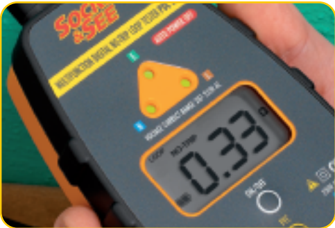
4 The PDL 310 showing a measured value of loop impedance
