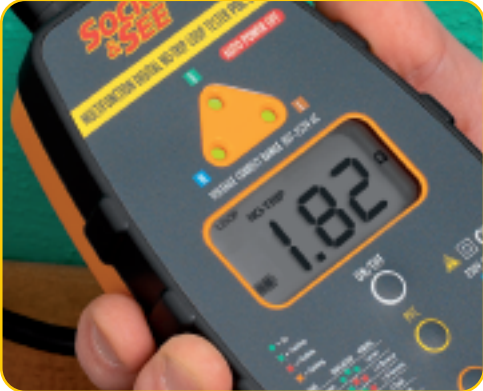
5 The PDL 310 showing a higher value of loop impedance.
