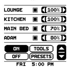
Press ON to turn the air-conditioning system On
