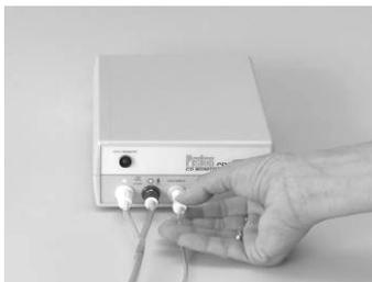
Connect the blue connector of the twin tubing to the blue coded socket indicated with the Flow meter label and the white connector to the white coded socket
