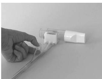
The disc filter of the gas sampling tubing prevents the device from the contamination
