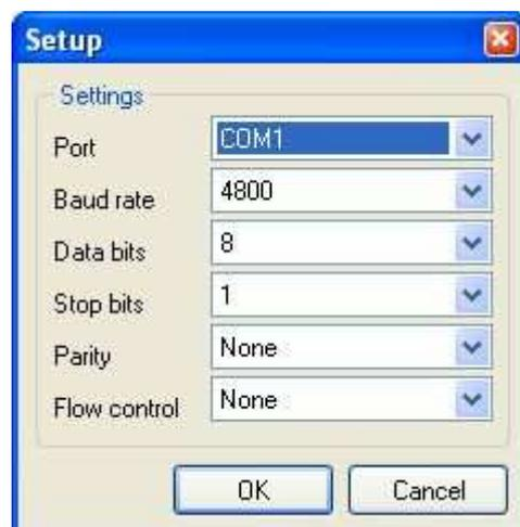
Select the appropriate PC port where the loading equipment is connected
