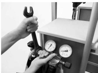
Regularly change the sealing ring of the gas cylinder
