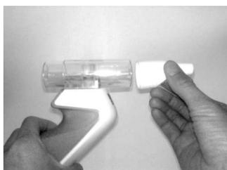
Connect one MPA-30 mouthpiece to bigger diameter end of the PinkFlow flow meter
