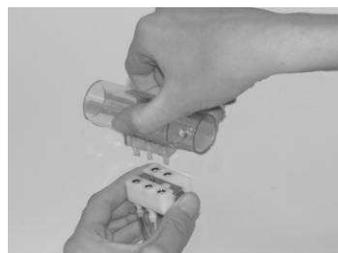
Connect the flow meter dock to a clean Pink-Flow flow meter. Push the metal release button to remove the PinkFlow flow meter from the docker.
