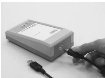
Connect the USB cable to the device and to the PC
