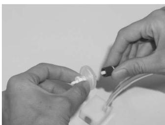
The disc filter of the pressure port prevents the device from the contamination
