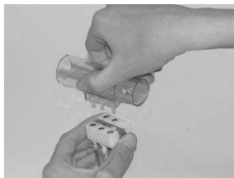
For the connection push the PinkFlow flow meter into the quick connector
