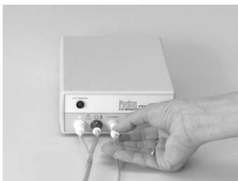
Connect the yellow connector indicated with the Gas sample label to the yellow coded socket
