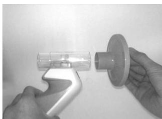
Connect one PBF-100MG bacterial and viral filter to bigger diameter end of the PinkFlow flow meter
