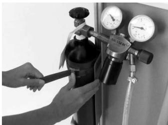
Place the gas cylinder to the PC cart and fasten it with the belt
