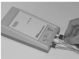
Connect the green connector of the nasal pressure tubing to the green coded socket
