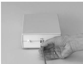
Connect the USB cable to the device and to the PC
