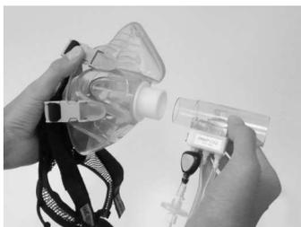
Push the smaller diameter side of the PinkFlow flow meter into the white adapter ring
