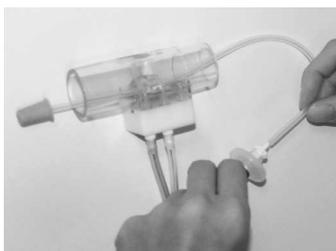
Connect the tubing of the Nasal probe to the barbed fitting of the disc bacterial filter
