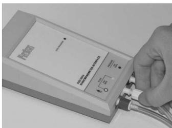
Connect the blue connector of the twin tubing to the blue coded socket indicated with the Flow meter label and the white connector to the white coded socket
