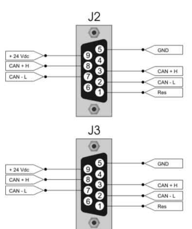
Is possible insert the TERMINATOR RESISTOR, connecting the PIN 1 and 2 of J2 or J3
